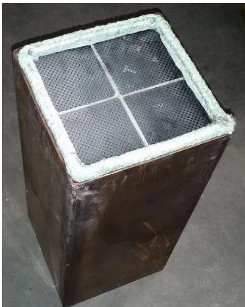
Image x Filter element with gasket attached
