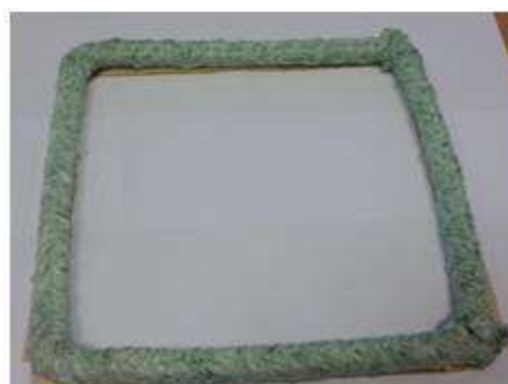
Image x Customised filter gasket
