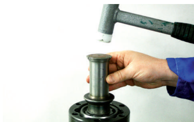
10. Carefully drive ball hub onto shaft until it reaches bottom position
