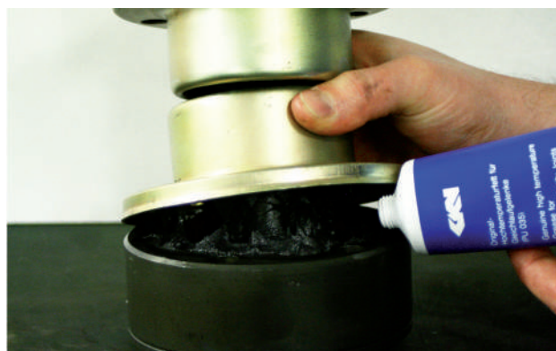
12. Fill inside of CV-joint with approx. half the grease supplied
