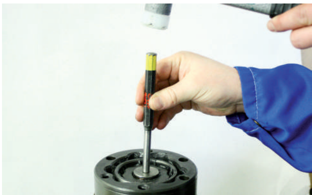
5. Carefully drive intermediate shaft out off CV-joint
